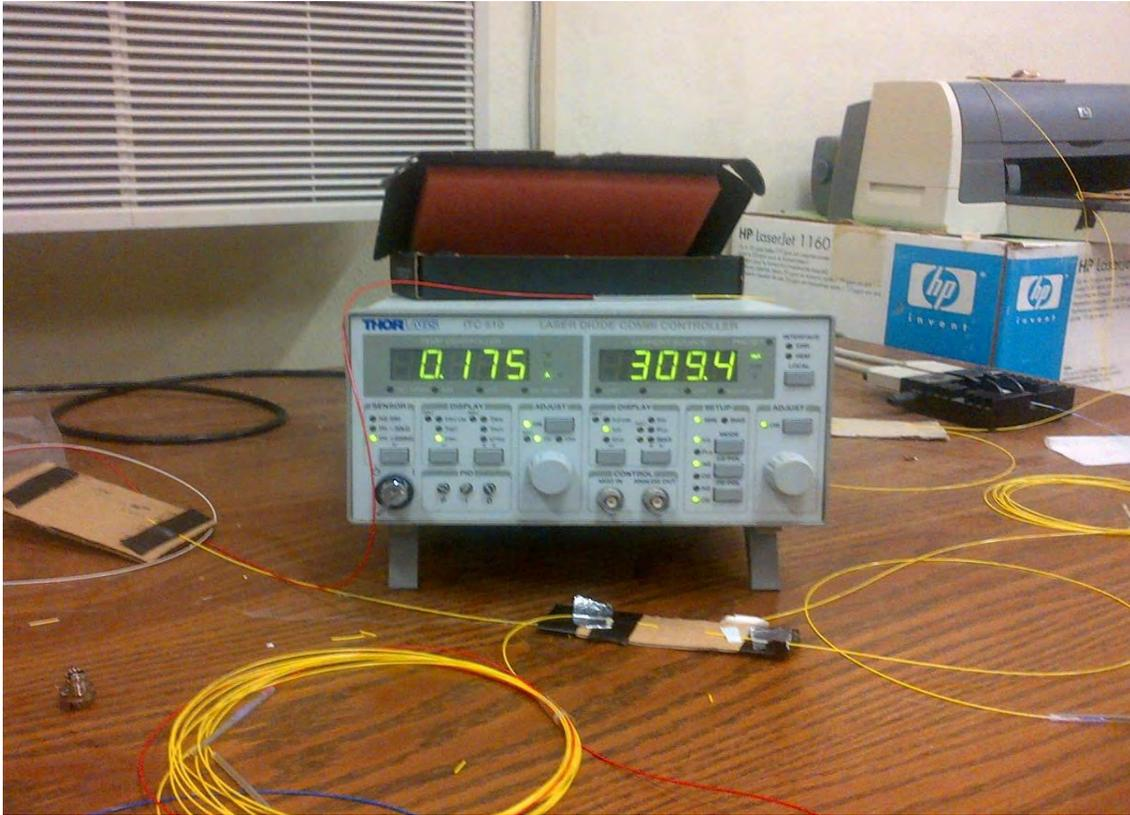
Figura 18 Laser ThorLabs ITC 510 Laser Diode Combi Controller (Laser a 950nm)
