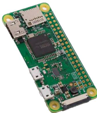
Figura 13. Raspberry Pi Zero W
